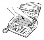
**5** Wind the film slightly (rotate the gear on the right side of the rear spool) so that there is no slack in the film. Make sure that both edges of the film wind onto the spool evenly.
